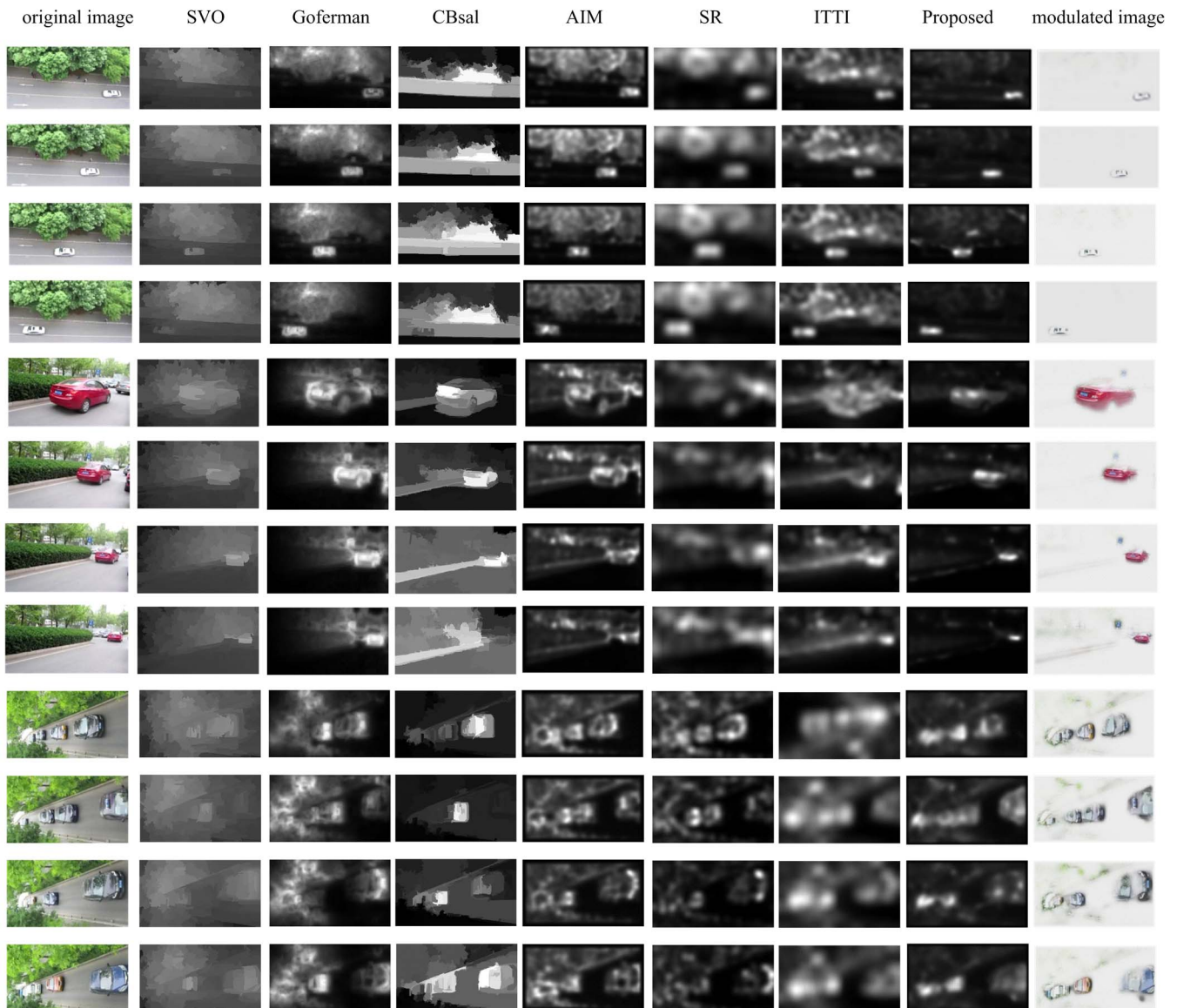
Figure 4 | Experimental results of the seven models tested with traffic images. The first column shows the original images; the second to eighth columns present the saliency maps obtained by SVO, Goferman's model, CBsal, AIM, SR, ITTI's model, and the proposed model, respectively. Images modulated by the corresponding saliency maps obtained by the proposed method are given in the last column. The original images are all taken by X.H. Wang with a digital camera Canon IXUS 125HS.
