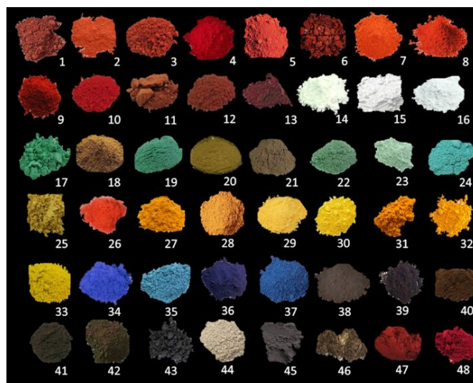
Figure 1. Set of 48 natural powdered pigments by Zecchi store collection. From 1 to 13, Red pigments: Hematite, Ercolano , Cinabrese , Carmine, Ochre, Dragon's blood, Coral, Red Lead, Alizarin, Cinnabar, Bolo , Jasper, Morellone ; from 14 to 16, White Pigments: White Lead, San Giovanni , White Bone; from 17 to 33, Earths (green and yellow pigments): Malachite , Campeggio , Chrysocolla, Aloe, Brazilwood, Jasper, Verdaccio , Verdigris, Arzica , Saffron, Turmeric, Yellow Ochre, Giallorino , Yellow Napoli, Gommagutta , Orpiment, Stil de grain; from 34 to 37, Blue pigments: Smalt, Azurite, Indigo, Lapis lazuli; from 38 to 43, Black Lamp, Ivory, Sepia, Bitumen, Vine Black, and Graphite; from 44 to 46: Vicenza Earth , Romana Earth , and Schist. Finally, the lake pigment, Gommalacca and Garanza , 47 and 48 respectively. The natural pigments reported in Italics are pure of Italian origin (e.g., Ercolano red is obtained from iron-deposits near Ercolano , Naples).
