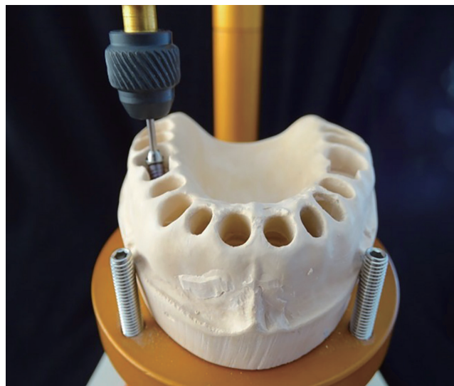
Fig. 1. Placing the implants on the gypsum model with the parallelometer.
