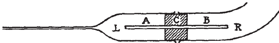
Figure 1. H_2O movement through cells of Nitella . (Top) Device for measuring fluid movement. A, Half of a single cell immersed in L; B, half of a single cell immersed in R; C, seal separating L and R; L, left aqueous compartment; R, right aqueous compartment. The compartments were insulated with a rubber pencil eraser or a piece of cork, anticipating later development of sucrose-gap preparations. (Bottom) Time course of movement of water from compartment L to R. The distance on the y axis indicates the movement of the water meniscus in the narrow neck of the capillary in compartment L. Curve 1 shows movement from L to R when the fluid in R is switched from H_2O to 0.4 M sucrose with distilled H_2O in L. Curve 2 shows movement in the reverse direction when solution R is replaced with 0.3 M sucrose, showing water flows from a more concentrated compartment to a more dilute compartment. In curve 3, compartment R is replaced with distilled water, bringing the system back to its original state. From Osterhout (1949).
