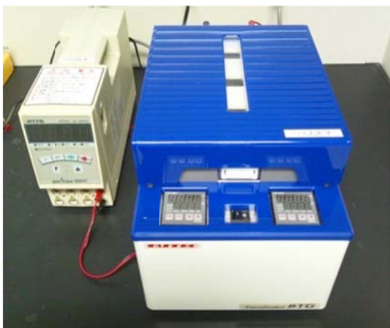
Fig. (1). Temperature gradient gel electrophoresis apparatus ( \mu TG; TAITEC, Saitama, Japan).
