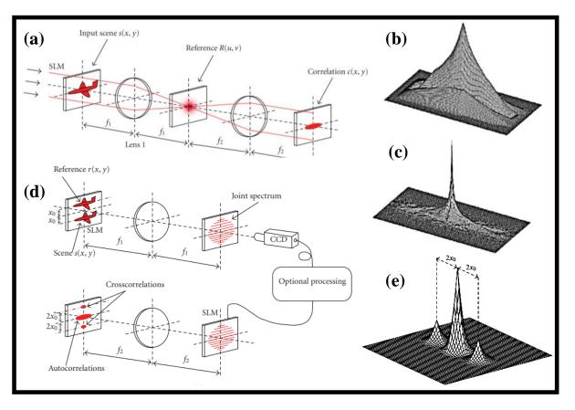
**Figure 1.** (a) Optical setup of basic 4-f correlator [22], (b) autocorrelation peak for a matched filter [22], (c) autocorrelation peak for a phase-only filter [22], (d) optical setup of JTC [22], (e) O/P plane of the JTC [22].
