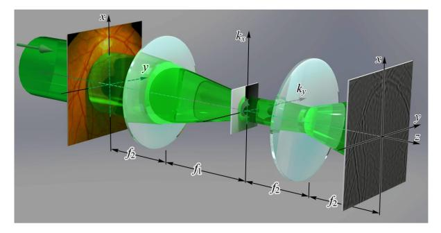
**Figure 2.** Illustration of the optical implementation of the radial Hilbert transform using the spiral phase plate as a spatial filter to contrast the image of the fundus vessels [51].
