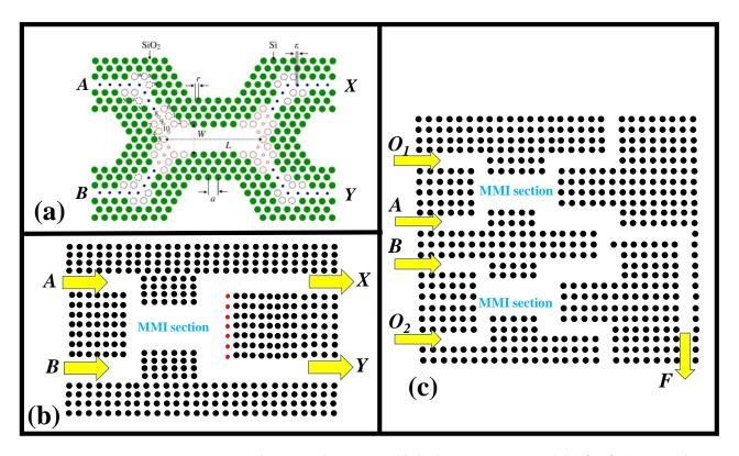
Figure 7. Schematic of OLGs established on MMI. Inspired by [146], (a) AND/XOR OLG, (b) XOR/XNOR, (c) AND and NOR OLGs. Inspired by [150].
