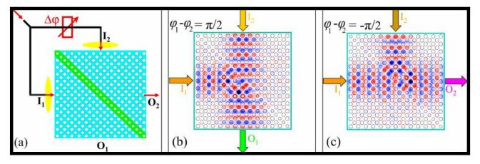
**Figure 6.** (a). The switch's schematic representation. On the I/P faces I<sub>1</sub> and I<sub>2</sub>, two beams with different phases collide. The computed steady-state field pattern of the E-polarized mode at 0.194 (a/ $\lambda$ ) when incoming beams propagate in the  $\Gamma$ -M direction in (b,c). The phase difference between the two incident beams is adjusted to  $\pi/2$  and  $-\pi/2$ , respectively, by the phase difference  $\varphi_1 - \varphi_2$  [143].
