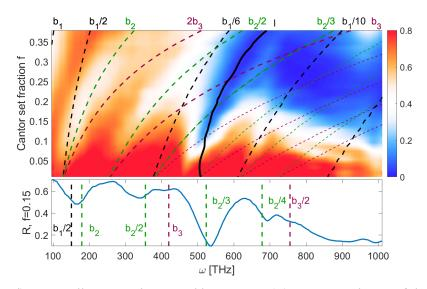
**Figure 3.** Reflection coefficient as a function of frequency and the Cantor set fraction f, for d = 0 and h = 45 nm. Black, green and magenta lines mark the plasmonic modes corresponding to first, second and third iteration structures.
