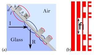
**Figure 1.** (a) Schematics of the considered plasmonic system, with propogation direction of incident (I) and reflected (R) waves. (b) First three iterations of Cantor set construction with structure length *l* and removed part fraction f = 1/3.
