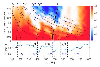
**Figure 4.** Reflection coefficient as a function of frequency and the Cantor set fraction f, for d = 45 nm and h = 90 nm. Black lines mark the island modes. Blue and magenta lines are the groove modes with and without low f correction, respectively.
