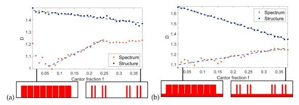
**Figure 6.** Calculated dimension of the reflection spectrum for (**a**) d = 0, h = 45 nm and (**b**) d = 45 nm, h = 90 nm. Insets: schematic of the structure.
