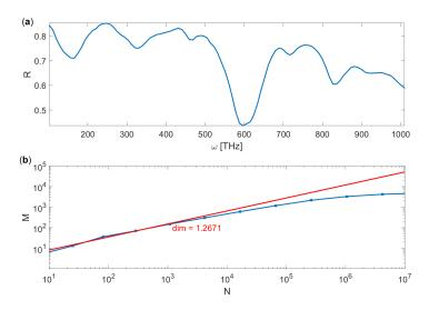
**Figure 5.** (a) Numerically calculated reflection coefficient for d = 0, h = 45 nm, f = 1/3. (b) The fractal dimension of the curve determined by fitting (red line), according to the Equation (7).
