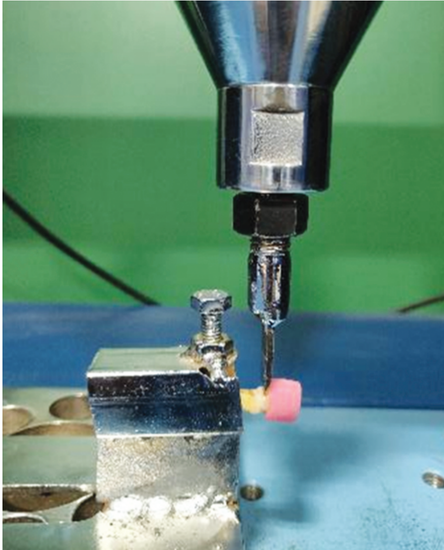
Fig. 2: Universal testing machine used to test the adhesive bond strength of the cement
