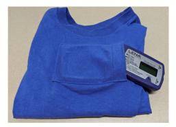
**Figure 4.** The Language Environment Analysis System (LENA Research Foundation, 2015) alongside the specially made t-shirt. The chest pocket secures the LENA throughout the day with a snap button.
