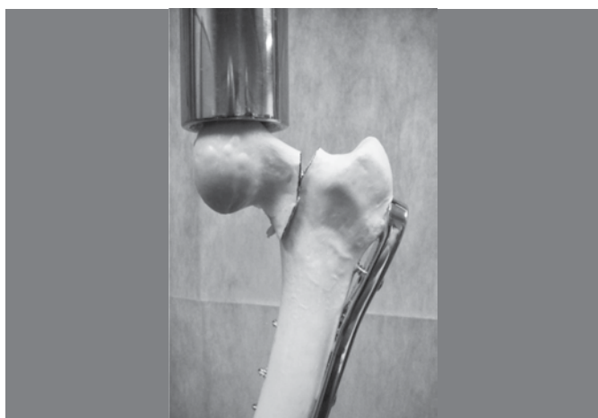
Figure 6. Image of the bone model used at the 10mm displacement assay (Step 2).
