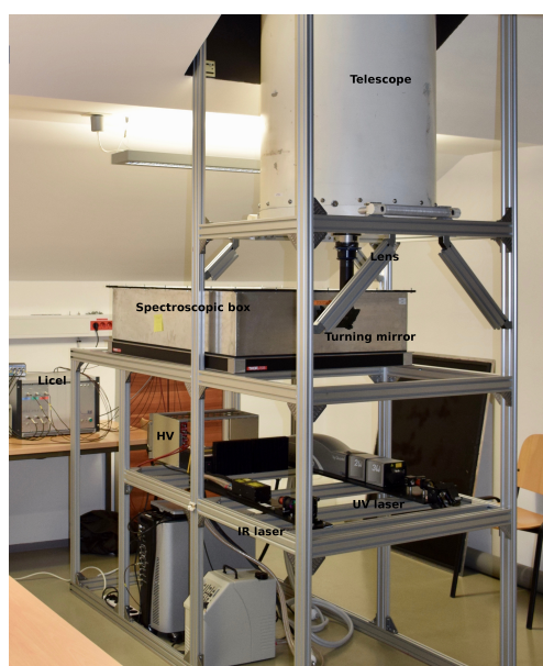
Figure 3. Assembled LiDAR system in its working environment at the Center for Atmospheric Research of the University of Nova Gorica in Ajdovščina. The atmosphere is accessed through a 1-m 2 rooftop borosilicate window with >85% light transmission in UV and IR and a remotely-controlled shutter. The telescope is mounted as close to the window as possible, leaving room for the spectroscopic filter and the transmitter below.
