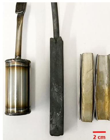
Figure 2. Photograph presenting a new sealed canister ( left ), a forged billet ( center ) and a cut-out sample ( right ).
