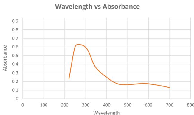
**Figure 4.** UV–visible spectrum for FeONPs synthesized using *Madhuca indica* plant extracts with 25 mM FeSO<sub>4</sub>.
