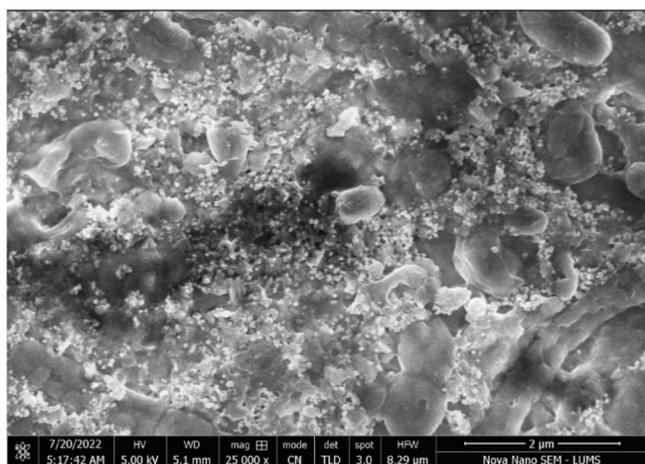
**Figure 6.** SEM image of green synthesized FeONPs at  $2 \mu\text{m}$  scale.
