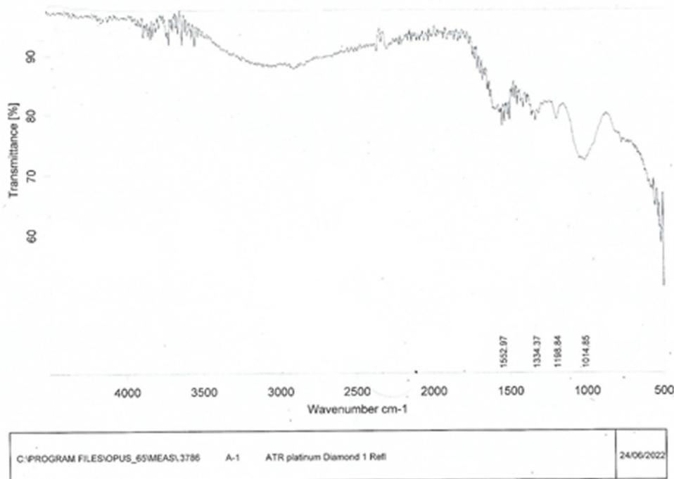
**Figure 5.** FTIR spectrum of Ferric oxide nanoparticles synthesized using the leaf extract of *Madhuca indica* and  $\text{FeSO}_4$ .
