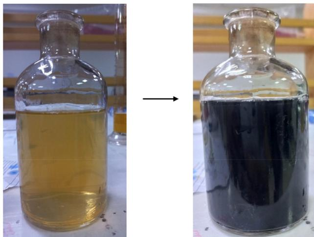
**Figure 3.** Color change indication of the solution mixture after the addition of FeSO<sub>4</sub> to the plant extract.
