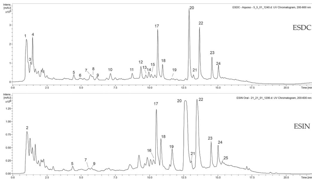
Fig. 7. HPLC-PDA-ESI-IT-MS<sup>n</sup> analysis of dry extracts ESDC and ESIN.
