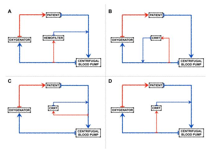
Figure I (A) In-line Hemofilter. (B) Full RRT circuit into the ECMO circuit: section of the circuit under positive pressure. (C) Full RRT circuit into the ECMO circuit: section of the circuit under negative pressure. (D) Full RRT circuit into the ECMO circuit: section of the circuit under positive and negative pressure.
