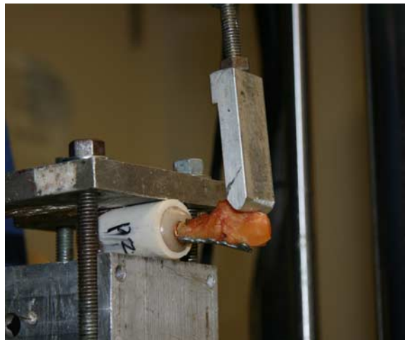
FIGURE 3. Biomechanical testing set up on the MTS machine. The metacarpal potted in a polyvinyl chloride pipe is stabilized while the hamate is loaded in extension. full color online
