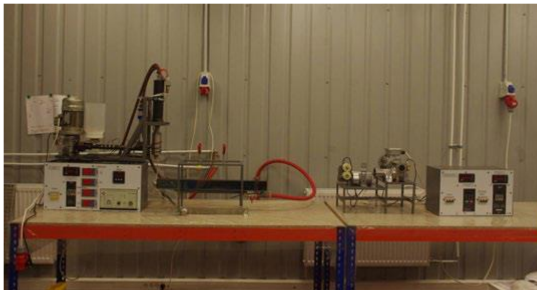
Figure 2. Laboratory extruder with ultrasonic melt treatment.
