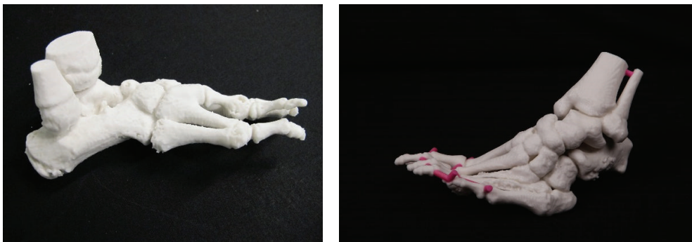
FIGURE 2: Preoperative model of ankle made by binder jetting with monochrome and with colors.
