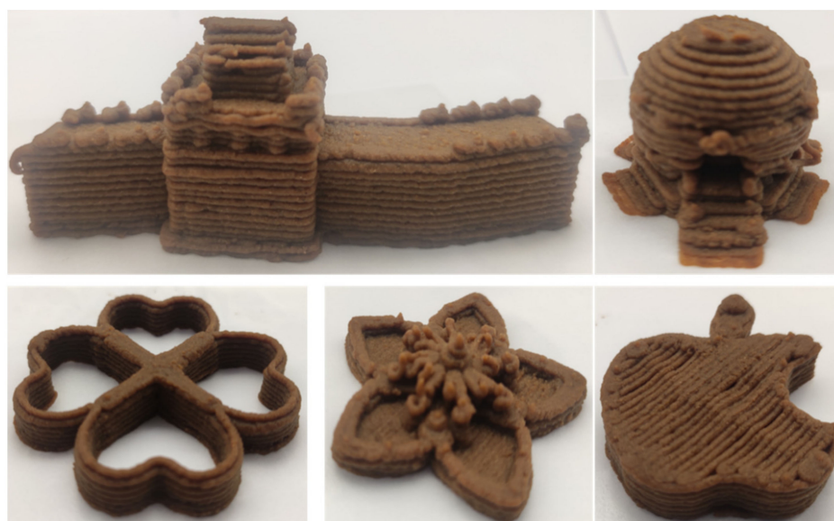
Figure 8. Pictures of 3D printed representative samples using XG-0.6% containing ink.
