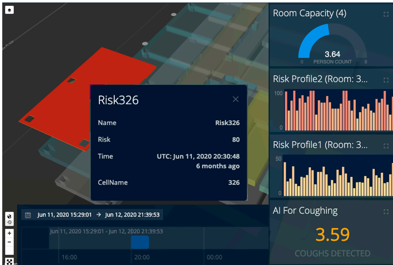
Figure 15. Risk profiles for room 326 over the period of 40 min from 20:00 to 20: 40 p.m. on 11 June 2020: Two gadget shows risk profiles and each bar demonstrate calculated risk for every minute.
