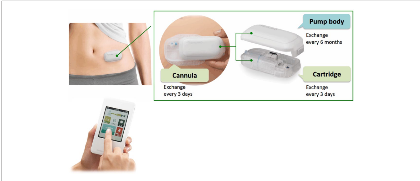
Figure 1. Components of the pump system: pump (above) and controller (below).
