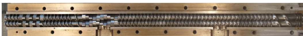
Figure 1. The appearance of an open plasticizing system of an extruder with processing screws.
