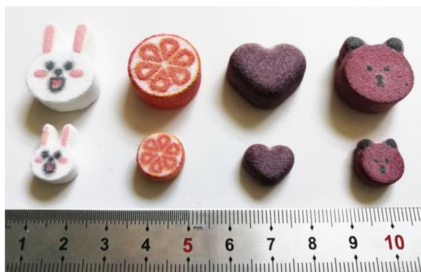
Fig. 8 – 3D printed cartoon tablets with different strengths. (A): 1000 mg strength; (B): 250 mg strength.
