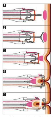
**Figure 1** Schematic illustration of an EFTR\* with FTRD<sup>®</sup> (www. ovesco.com). (1,2) Positioning on resection site with endoscope; (3) Grasping of marked tissue and drawing into cap with FTRD<sup>®</sup> grasper; (4) Application of the over-the-scope clip; (5) Snare closing and resection of tissue
