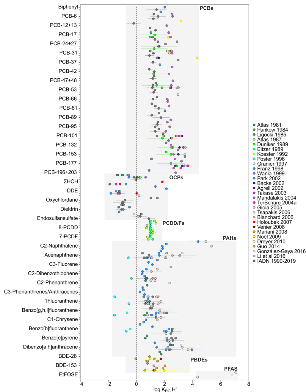
Figure 4. Predicted rain amplification of the fugacity ratio between rain and air given by the product of the rain–air (gas phase) partition constant and the dimensionless Henry's law constant ( f_w/f_G = K_{RG}H' ) for various families of organic pollutants. The results shown are the mean and the standard deviation of \log K_{RG}H' .
