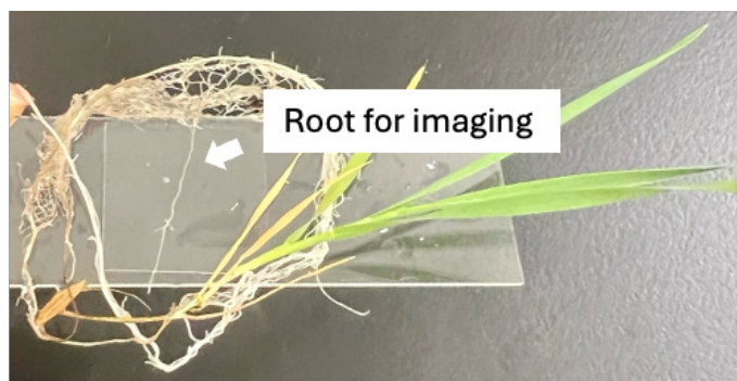
Figure 3. Arrangement of the root on the glass slide for confocal imaging
