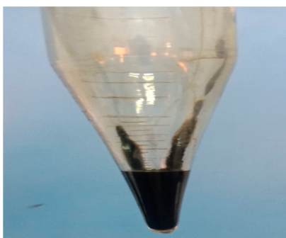
Figure 6. Asphaltene residue after the second centrifuge run with heptane.
