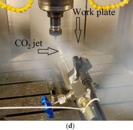
Figure 1. The experimental setup: (a) the work plate, cutter, and force plate; (b) milling under evaporative cryogenic cooling; (c) the side- and end-mill cutter used in the experiments; and (d) milling under throttle cryogenic cooling.
