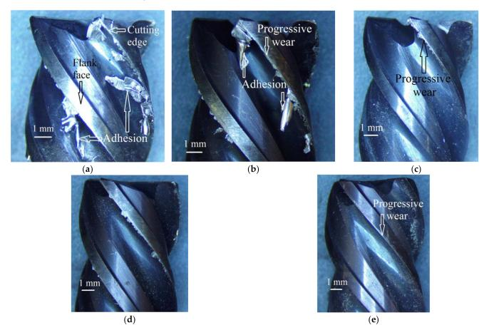
**Figure 3.** Micrographs of the milling cutters used in the following runs: (a) coolant = dry,  $V_c = 150 \text{ m/min}$ ; (b) coolant = evaporative, flow rate = 0.2 kg/min,  $V_c = 200 \text{ m/min}$ ; (c) coolant = evaporative, flow rate = 0.6 kg/min,  $V_c = 200 \text{ m/min}$ ; (d) coolant = throttle, flow rate = 0.4 kg/min,  $V_c = 200 \text{ m/min}$ ; and (e) coolant = throttle, flow rate = 0.6 kg/min,  $V_c = 200 \text{ m/min}$ ;  $V_c = 200 \text{ m/min}$ ;
