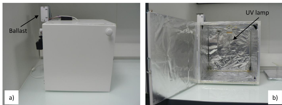
Fig. 1. Home-made UV irradiation chamber, lined inside of aluminum foil, equipped with UV lamp (after light bulb was removed) and a ballast for lamp operating. (a) Outside view, (b) Inside view.
