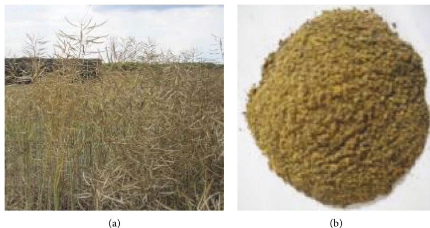
FIGURE 1: Rapeseed residual biomass: (a) straw, leaves, and pods; (b) residual rapeseed biomass ground and sieved to the particle size of \leq 0.25 mm.
