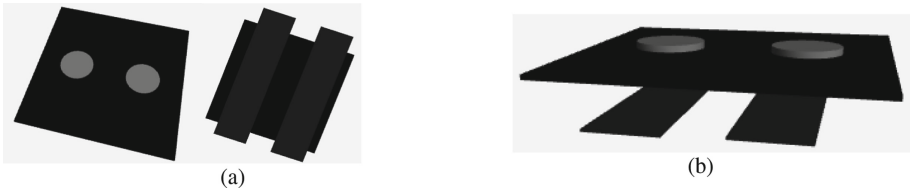
Fig. 5. Base developed to fix the labellum. (a) Top and bottom view. (b) Side view.
