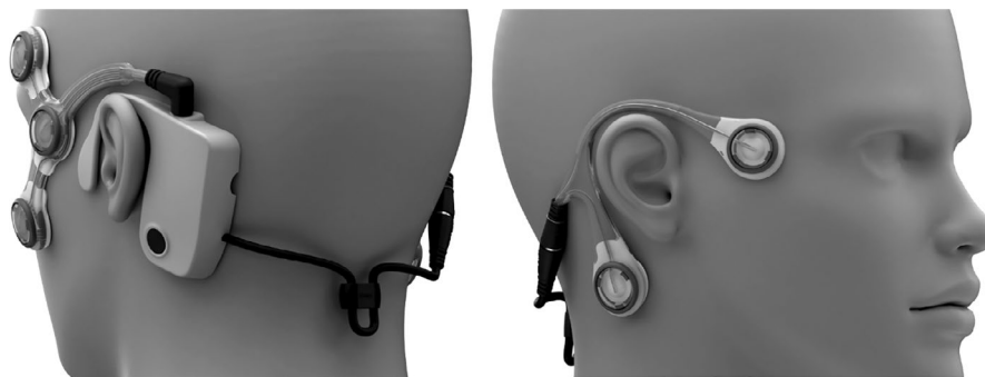
FIGURE 1 A depiction of the CAVA ® device when worn on the face. A reusable logging module sits behind the left ear, and two single-use electrode mounts attach to the face. The mounts contain five ECG electrode pads, facilitating the capture of both horizontal and vertical eye movements. An “event marker” button on the logging module allows patients to log events of interest (eg the onset of dizziness). The device also captures head movement by way of a 3-axis accelerometer
