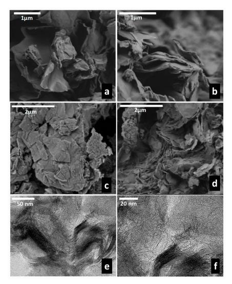
**Figure 11.** FE-SEM images of the pristine Co-LSH (**a**,**b**), and the Z-LSH\_ cppt (**c**) and Z-LSH\_ie (**d**) biohybrids. TEM images of Z-LSH\_ie biohybrid (**e**,**f**).
