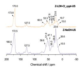
Figure 6. Solid state <sup>13</sup>C NMR spectra of Z-NaOH-US and the Z-LDH-Cl\_cppt-US biohybrid.
