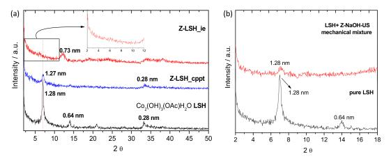
**Figure 8.** (a) XRD patterns of pristine Co-LSH, and Z-LSH\_cppt and Z-LSH\_ie biohybrids prepared by co-precipitation and ion-exchange methods, respectively; (b) XRD patterns of pristine Co-LSH containing acetate anions and the mechanical mixture based on Co-LSH and Z-NaOH-US.
