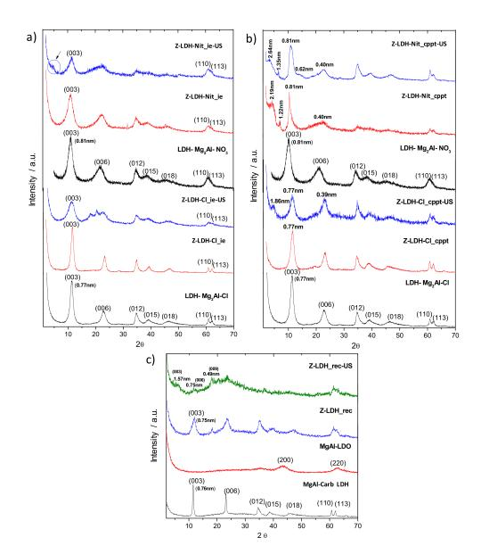
**Figure 4.** XRD diffractograms of Z-LDH biohybrids prepared by the (**a**) ion-exchange, (**b**) co-precipitation, and (**c**) reconstruction methods from zein dissolved in 0.1 M NaOH with and without US (60 kJ).
