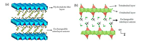
**Figure 1.** Schematic representation of the crystal structure of (**a**) typical layered double hydroxide (LDH) and (**b**) layered single hydroxide (LSH) layered solids.
