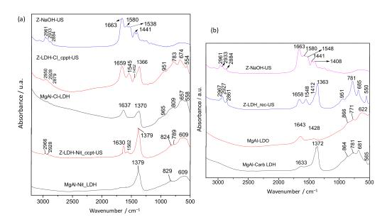
**Figure 5.** FTIR spectra in the 3200–500 cm<sup>-1</sup> region of LDH and Z-LDH biohybrids prepared by (**a**) co-precipitation and (**b**) reconstruction from zein dissolved in 0.1 M NaOH under US.
