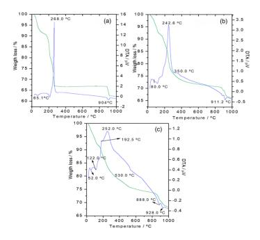
**Figure 10.** TG and DTA curves of (**a**) Co-LSH, and (**b**) Z-LSH\_cppt and (**c**) Z-LSH\_ie biohybrids carried out under air flow.
