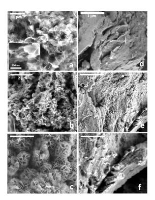
**Figure 7.** FE-SEM images of (**a**) MgAl–Cl, (**b**) MgAl–Nit and (**c**) MgAl-Carb LDH, as well as the (**d**) Z-LDH-Cl\_cppt-US, (**e**) Z-LDH-Nit\_cppt-US, and (**f**) Z-LDH\_rec-US materials.
