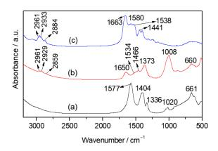
**Figure 9.** FTIR spectra in the 3200–500 cm<sup>-1</sup> region of pristine (**a**) Co<sub>2</sub>(OH)<sub>3</sub>(CH<sub>3</sub>COO)-LSH, the (**b**) Z-LSH\_ie biohybrid. and the (**c**) Z-NaOH-US.
