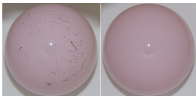
Figure 3. Head of CoM bearing (left) and CoC bearing (right).
