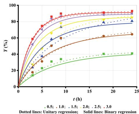
Fig. 2 Experimental data versus fitted lines of  $Y$  for lipase-catalyzed esterification of LA and methanol at different  $R_m$ . Enzyme loading: 10 g L<sup>-1</sup>; temperature: 303.15 K.
