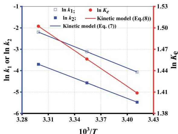
**Fig. 4** The fitting of rate/equilibrium constant with temperature.
