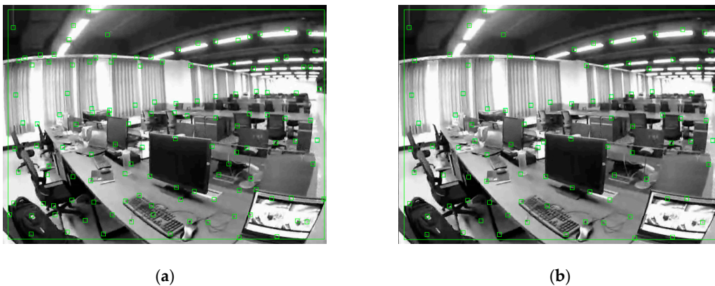
Figure 3. Feature points extraction in the grayscale image: (a) Original features from accelerated segment test (FAST) corner points distribution; (b) FAST corner points distribution after sparse processing.
