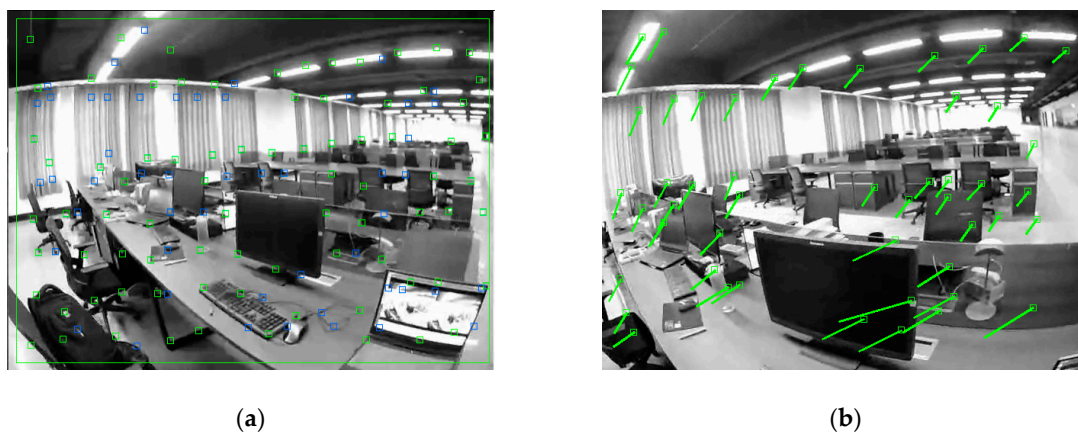
Figure 4. (a) FAST corner points distribution managed by the gridded map strategy; (b) Feature points tracked by the optical flow method.
