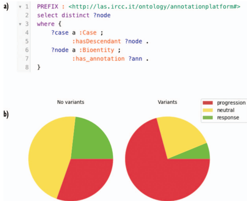
Figure 4. (A) A SPARQL query for retrieving annotated nodes. In the very first part, a ‘PREFIX’ is declared as a shorthand for local URIs. The pattern described in the ‘WHERE’ clause asks GraphDB to get all the annotated nodes. In line 2, the projection clause selects distinct nodes. (B) Response fractions in trees with no variants in the genes panel (on the left) and with one or more variants (on the right). Cases harboring variants in the panel are less sensitive to cetuximab.
