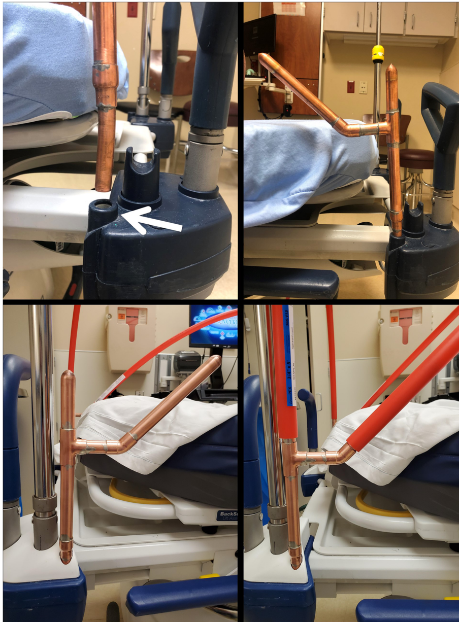
Fig. 3 Mounting of the copper posts and PEX tubes to commonly used patient beds in the emergency department. The posts are inserted to the bed through the \frac{3}{8} in. (1 cm) diameter connecting coil tube (arrow in upper left panel). The PEX tubes are inserted to the receiving ends of the copper posts
